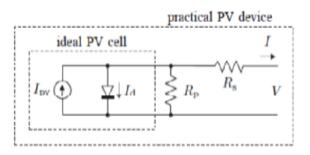
**Fig: 1.** Single-Diode Model of the Theoretical PV Cell and Equivalent Circuit of a Practical PV Cell
