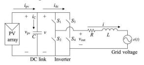
Fig: 3. Equivalent Circuit Diagram of Single-Phase Grid-Connected PV System
