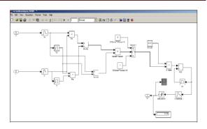
Fig: 6. Model for MPPT: Simulink Model for P&O Algorithm
