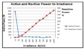
Fig: 8. Active and Reactive Power Variation at Inverter Output
